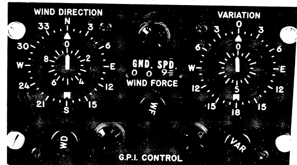
C-1316/ASN-6 RIGHT CONSOLE CONTROL PANEL
